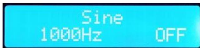
*Setting a sine wave signal with a frequency of 1 kHz. (© 2018 Jos Verstraten)*
